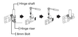
Attach the hinge on the bottom left side of the refrigerator where bolts were previously removed in step 6.
